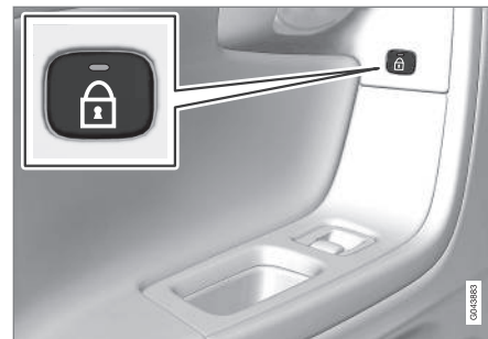
The indicator light in the button is on when the door is locked
