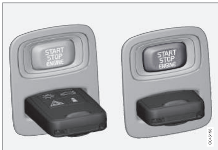
Ignition slot with remote key inserted ( see page 86 for more information on ignition modes)
