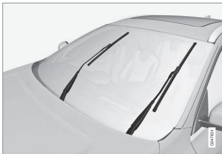
Wiper blades in service position
