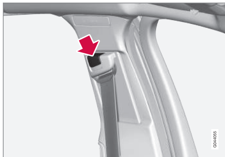
Adjusting seat belt height
