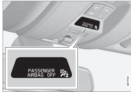
Occupant Weight Sensor (OWS) indicator light
