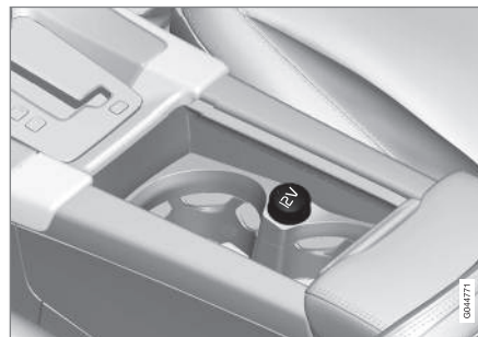
12-volt socket in the front tunnel console
