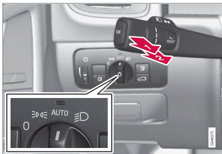
Headlight switch and steering wheel lever
