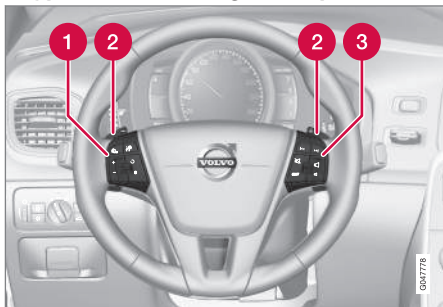
Steering wheel keypads and paddles*
