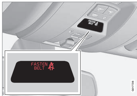
Seat belt reminder light in ceiling console
