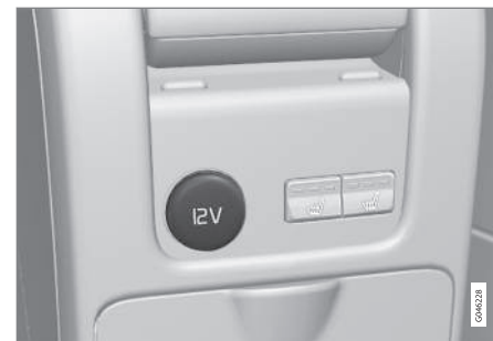
12-volt socket in the rear center console
