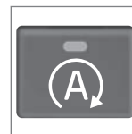
Start/Stop button on the center console
