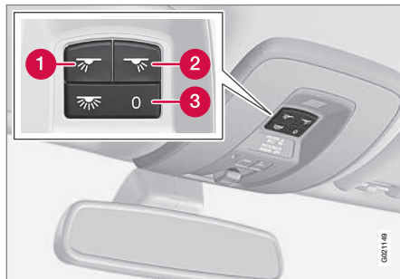
Light switches, front roof lighting
