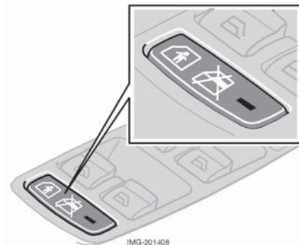
Electrical lock for opening the rear door and window
