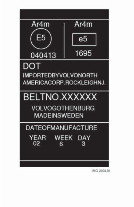
Marking on seat belts with seat belt tensioners
