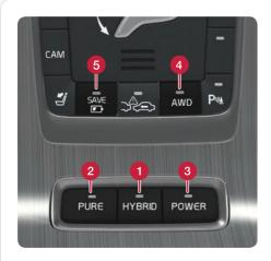
The car is powered by two motors - one electric and one diesel. Different drive modes can be selected. It is not possible to select the "wrong" drive mode - the car returns to the HYBRID mode if certain conditions are not met. The lamp in the hybrid button will then illuminate.
