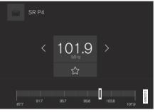
Searching manually makes it possible to find and tune to stations that are not on the automatically compiled list of the strongest stations in the area.
