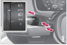
Steering wheel stalk switch with rotating ring.
