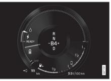
The driver display indicates charging during electric motor braking.
