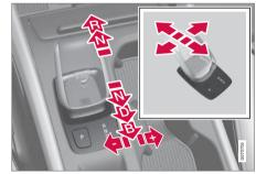
Overview of gear lever and gear positions.
