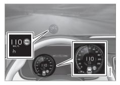
The previous illustration shows that the adaptive cruise control is set to maintain 110 km/h (68 mph) and that there is no vehicle ahead to follow.
