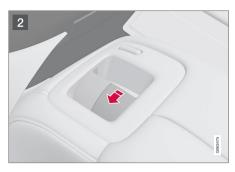
For cars without electronic folding, the outer head restraints are folded manually using the inner control on the upper side of the seat; see figure 2.
