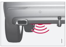
The sensor is located on left of centre in the bumper<sup>14</sup>.
