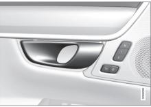
Opening handle for alternative unlocking in the side door<sup>11</sup>.
