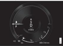
The hybrid gauge shows in different ways the relationship between how much power is being taken from the electric motor and how much power is available.
