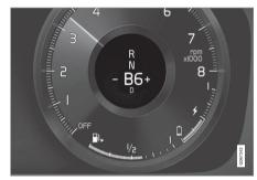
Gear shift indicator in the driver display<sup>5</sup>.
