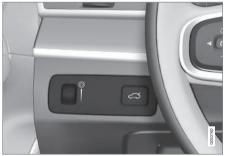
Thumbwheel (to left) for adjusting interior brightness.
