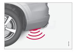
To activate opening or closing with a foot movement on a car equipped with skid plate, the kicking motion is made from the side of the car. One of the car's remote control keys must be within range (approx. 1 metre (3 feet)) for opening and closing to be possible.
