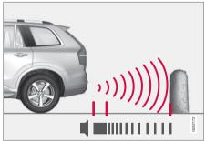
The warning signal has a constant tone at less than approx. 30 cm (1 ft) from an obstacle.
