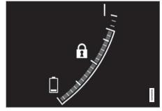
The ft symbol in the hybrid battery gauge indicates that the Hold function is activated, and the **f** symbol indicates that the Charge function is activated.
