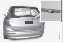
The backwards-facing camera is fitted above the registration plate.
