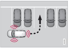
Principle for reversing into perpendicular parking.
