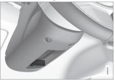
Lever for steering wheel adjustment.
