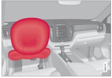
Steering wheel airbag and knee airbag  $^{\rm 1}$  on the driver's side in the front seat.
