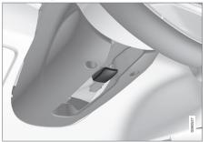
Lever for steering wheel adjustment.
