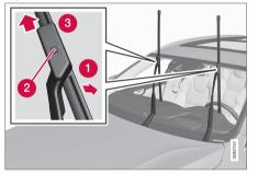
Fold up the wiper arm when it is in service position. Service position is activated/deactivated via the function view in the centre display when the car is stationary and the windscreen wipers are not on.
