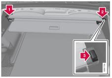
Insert one of the cargo cover's end pieces in the recess in the side panel in the cargo area. 2 Then insert the other end piece in the recess in the side panel on the opposite side.
