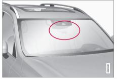
The marked area must be cleaned regularly and kept free from stickers, objects, shade film, etc.
