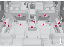
Storage compartment in door panel, cup holder\* in centre seat backrest, storage pocket\* on front seat backrest, electrical sockets in tunnel console, as well as storage compartment under seat.
