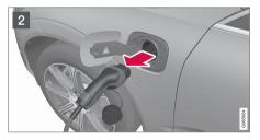
2 Unplug the cable from the car's charging input socket and close the hatch.
