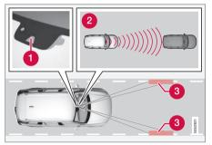
The camera and radar unit measures the distance to the vehicle ahead and detects side markings.
