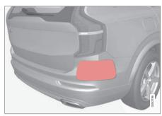
Location of rear radar units. Keep the surface indicated clean - on both the left and right-hand sides of the car.
