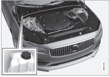
Coolant expansion tank, left-hand drive car.
