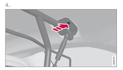
Insert the supplied screw and tighten using the supplied 6 mm Allen key. Repeat on the other side. Recommended tightening torque: 20 Nm (15 foot-pounds).
