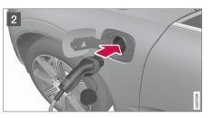
2 Open the charging hatch. Remove the charging handle's protective cover and then press the handle the whole way into the socket for the car.
