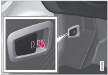
Pull the handle near the foot pedals to release the bonnet from its fully closed position.
