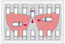
Examples of areas where CTA can assist the driver to detect obstacles during reversing.
