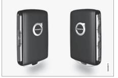
The remote control key has four buttons - one on the left-hand side and three on the right-hand side.
