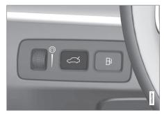
Long press on the instrument panel's A button. Keep it depressed until the tailgate starts to open.
