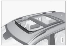
The panorama roof has a wind deflector that is raised when the panorama roof is in the open position.
