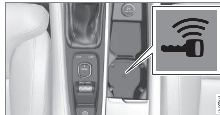
Backup reader's location in the tunnel console.
