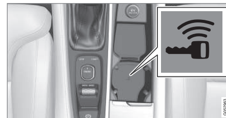
Backup reader's location in the tunnel console.
