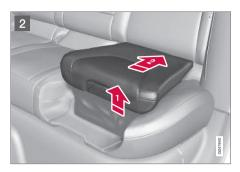
Lift the booster cushion up at the front edge and press it back against the backrest to lock.
