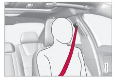
Correctly fitted seatbelt.
