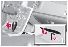
If the car cannot be driven, e.g. due to a flat starter battery, the gear selector must be moved from the **P** position so that the car can be moved.
