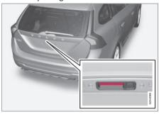
Rubber plate with electrical contact.
