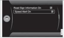
The driver can opt to receive a warning when the applicable speed limit is exceeded by 5 km/h (5 mph) or more. This warning is given by the symbol showing the applicable maximum speed temporarily flashing when this speed is exceeded. The function can be activated/deactivated in the menu system MY CAR. For a description of the menu system, see MY CAR (p. 115).
