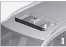
The sunroof has a wind deflector that is folded up when the sunroof is in the open position.
