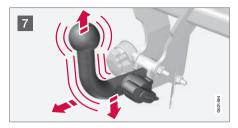
Check that the towbar is secure by pulling it up, down and back.
