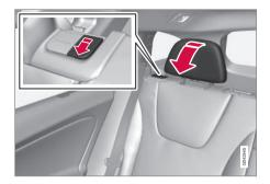
Pull the locking handle closest to the head restraint to fold the head restraint forward.
