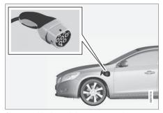
Charging cable plug and charging input socket.
