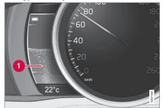
When the electric motor generates power for the hybrid battery, bubbles are shown in the hybrid battery gauge - see Foot brake (p. 279).
