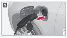
Remove the charging handle's cover and then connect the handle to the car.
