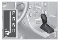
**D**: Automatic gear positions. +/-: Manual gear positions. **S**: Sport mode\*4.
