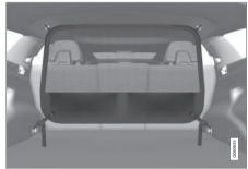
A safety net prevents loads or pets from being thrown forward in the passenger compartment in the event of sudden braking. For safety reasons, the safety net must always be correctly fastened and secured.
