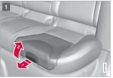
Pull the handle forward and up in order to release the booster cushion.
