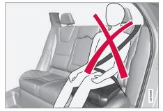
Incorrect positioning, the seatbelt must not be placed beneath the shoulder.
