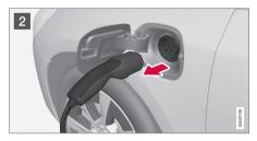
Unplug the cable from the car's electrical input socket, refit the charging input socket's cover and close the hatch, see Charging the hybrid battery - preparations (p. 300).
