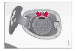
The LED lamps show the current status while charging is in progress. The white, blue, red and yellow lamps are activated when the passenger compartment lighting is switched on - they remain switched on for a while after the passenger compartment lighting has been switched off.
