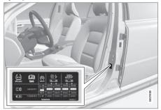
The tyre pressure label on the driver side's door pillar (between frame and rear door) shows the tyre pressures for the car's recommended tyre dimensions. This is also specified in the tyre pressure table, see Tyres - approved tyre pressures (p. 423).
