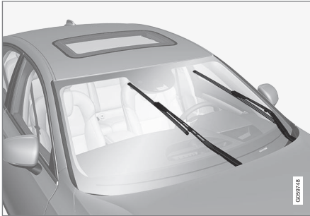
Viskerblade i servicestilling.
