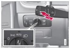
Headlight switch and steering wheel lever
