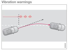
LKA provides vibrations in the steering wheel and steering assistance<sup>11</sup>.
