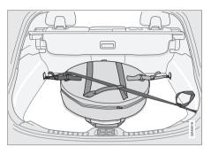
Turn the handle on the spare wheel bag out toward you. Secure the stitched strap hooks in the front loading eyelets. Secure the long strap in one of the front loading eyelets, wrap the strap diagonally over the spare wheel and through the upper handle. Secure the short strap on the long strap. Secure in the rear loading eyelet and tighten.
