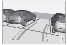
The lines on the screen are projected as if they were a path on the ground behind the vehicle and are directly affected by the way in which the steering wheel is turned. This enables the driver to see path the vehicle will take, even if he/she turns the steering wheel while backing up.
