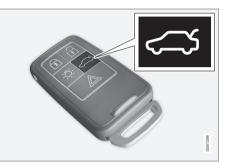
Tailgate unlock button on the remote key
