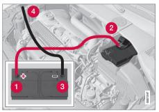
Connecting the jumper cables
