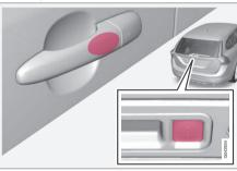
Models with keyless drive have a pressure-sensitive area on the outside door handles and a rubber-covered button next to the tailgate opening control
