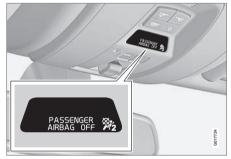
Occupant Weight Sensor (OWS) indicator light
