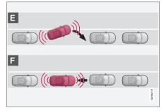
After the vehicle has backed into the parking space, its position in the space has to be adjusted by driving slightly forward and backing up.
