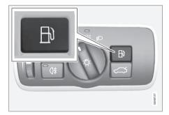
With the ignition switched off, press and release the button on the lighting panel to unlock the fuel filler door. Please note that the fuel filler door will remain unlocked until the vehicle begins to move forward. An audible click will be heard when the fuel filler door relocks.
