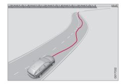
A camera monitors the painted lines marking the lane in which the vehicle is traveling and compares the direction of the road with the driver's movements of the steering wheel. The driver is alerted if the vehicle does not follow the lane smoothly.
