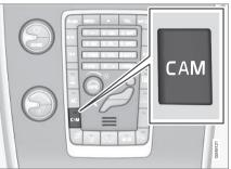
PAC is activated when the gear selector is moved to **R** if the system is selected in the **MY CAR** menu system or by pressing the **CAM** button in the center console. See My Car – introduction (p. 74) for a description of the menu system.
