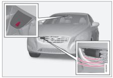
Camera and radar sensor<sup>6</sup>.
