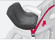
Pull out the shoulder section of the seat belt
