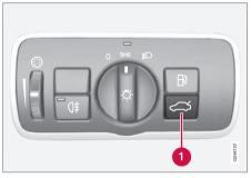
Press the button on the lighting panel (1) to unlock (but not open) the tailgate.
