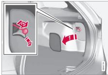
1. Open the side hatch in the cargo area (on the same side as the fuel filler door).
