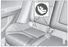
Symbols on the seat back upholstery mark the ISOFIX/LATCH anchor positions as shown. To access the anchors, kneel on the seat cushion and locate the anchors by feel. Always follow your child seat manufacturer's installation instructions, and use both ISOFIX/ LATCH lower anchors and top tethers (p. 56) whenever possible.
