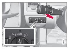
Models with an analog instrument panel When AHB is activated, the C symbol will illuminate in the instrument panel. The high beam indicator ( O) in the instrument panel will also illuminate when the high beams are on.
