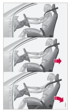
In the event of a rear-end collision, the hinges and brackets of the front seat backrests are designed to change position slightly to allow the backrest/head restraint to help support the occupant's head before moving slightly
