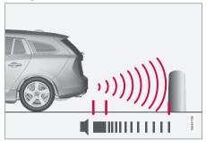
The distance monitored behind the vehicle is approximately 5 ft (1.5 m). The audible signal comes from the rear speakers.
